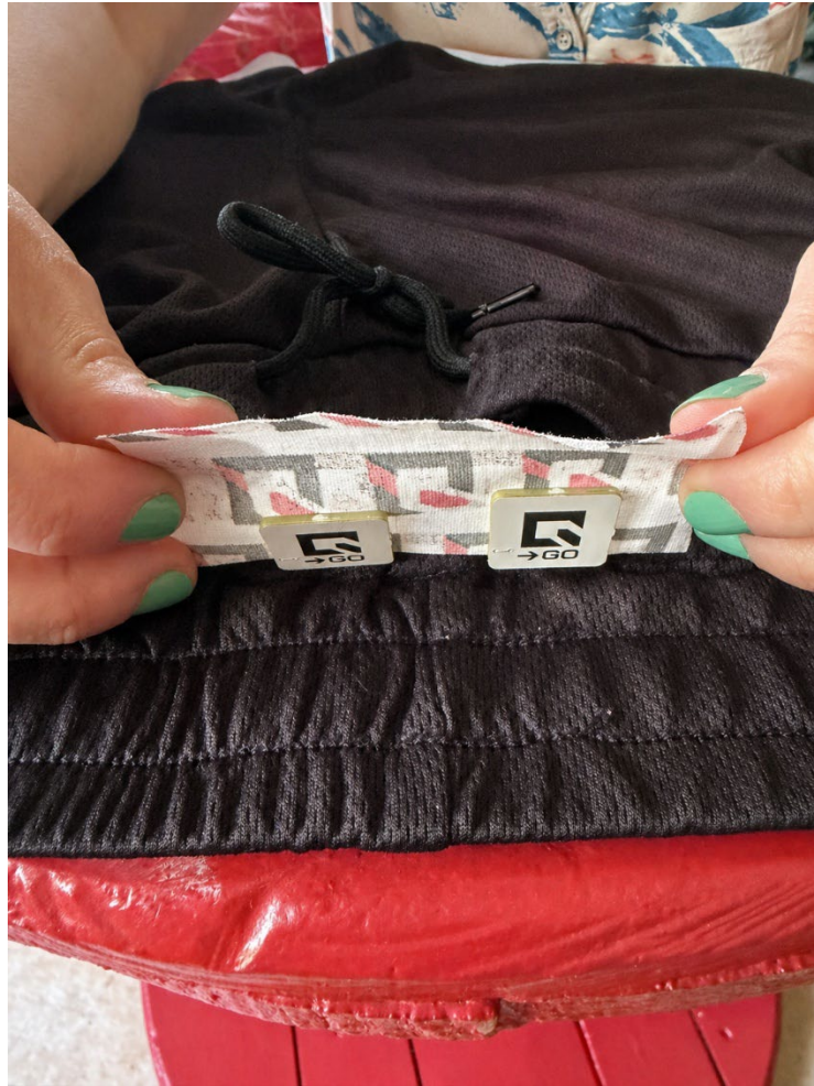
Q-Go circuits glued inside the shorts, back, logo against the fabric
